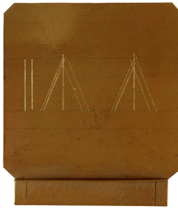
(b) Plate with inscribed pair of letter-forms prior to cutting parts from each letterform, with rectangle that will form 'lumière' (at left).
