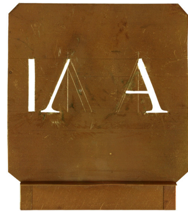
(c) Plate cutting and filing completed.
