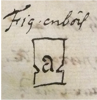
Figure 7. Gilles Filleau des Billettes, drawing of common stencil plate, from 'Imprimerie de Livres d'Eglise, Ecriteaux ou Sentences &c.', n. d. (c. late 1690s). The Newberry Library, Chicago, Wing MS oversize Z4029.225, p. 185 (detail).
