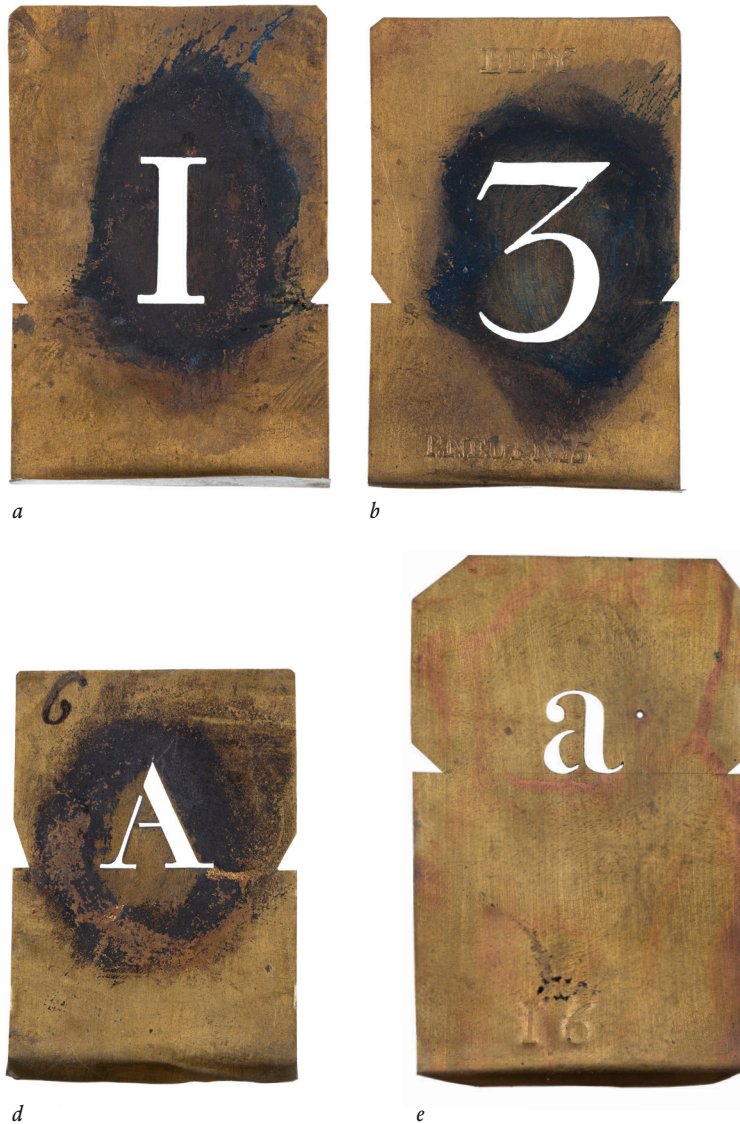
Figure 20. Stencils carrying size designations; brass, etched and filed.
