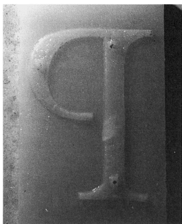
Figure 8. Wax cast of the simulated letter cavity.
