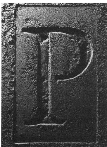
Figure 9. Impression of the wax cast in sand.
