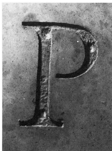
Figure 7. Simulated Roman letter cavity cut in limestone (approx. height 200 mm).
