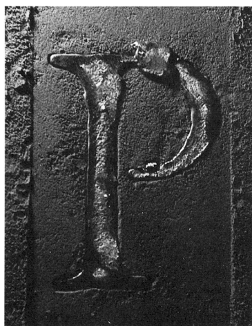
Figure 10. Infill made by pouring lead into the sand mould (note the uneven surface).
