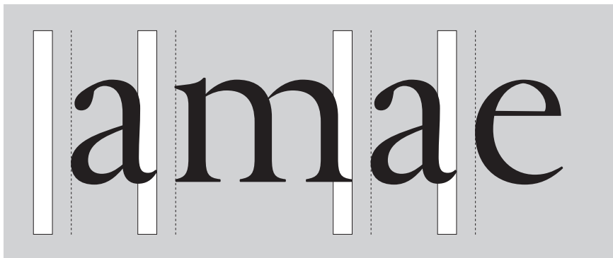
Figure 16. Inter-letter spaces. Des Billettes states that the inter-letter space should be measured between the extremities of adjacent letters, whatever those extremities are (serif, bowl, curve, etc.).
