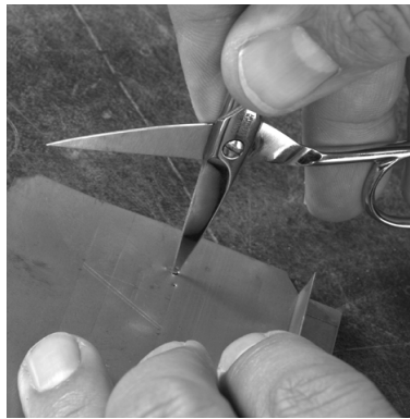
Figure 19. Rough cutting. A hole is first drilled through the thickest part (stroke) of the letter with the scissors. The letter is then cut by snipping outward from the hole and along the inscribed
