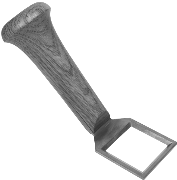
Figure 28. Holdfast ( patte ), brass (frame) and oak (handle), 62 mm (width of frame) × 150 (length of handle).
