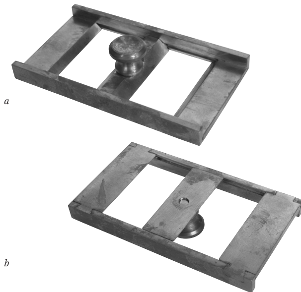
Figure 27. Sash-clamp ( sergent ), from above (a) and below (b), brass, 110 mm long × 61 wide × 10 high (excluding cursor button).
