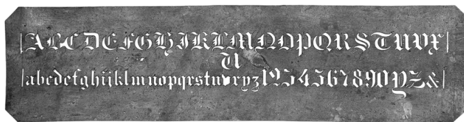
Figure A4.6. Stencil plate with complete character set, maker not known, probably French, c. first half of the 19th century, brass, etched, 50×195 mm. Stencil alphabets and numerals used by architects, engineers, and surveyors were also typically arranged horizontally on several plates. See Kindel (2010).
