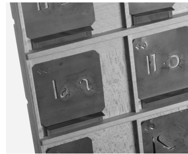
Figure 25. Lettercase (detail), compartments with stencils. The lower ledge of the compartment protrudes sufficiently to provide a secure rest for the stencil, but not so far that it interferes with picking up the stencil by its foot (handle).
