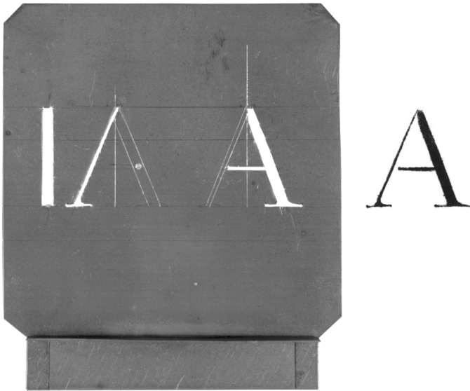
Figure 20. Rough cut, and stencilled proof.
