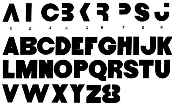
Figure A4.13. Specification drawing, Ezekiel B. Foster, US Letters Patent no. 4045 (1845). 'The nature of my invention consists in forming all the letters of the alphabet in stencil painting and printing by means of nine characters by changing, reversing and combining the said characters. Thus making nine characters to answer the place of twenty seven letters, in the operation of which the letters are made more perfect – leaving no spaces or interstices to be filled up after the brush has passed over the stencil as in the present mode, or mode now in use.' Foster included instructions for how each letter should be made, for example: 'X is formed by no. 5 as represented and a reversed impression annexed.'
