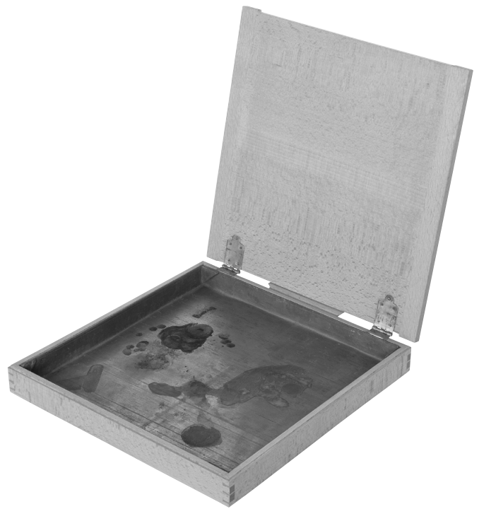
Figure 29. Ink box, beech, brass (hinges), lead (lining), 300 mm × 300 × 45 (closed). Simonneau illustrates the box with a lid, though Des Billettes makes no mention of it.
