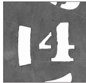
Figure A4.29. Stencil disk, made by New York Stencil Works, based on US Letters Patent no. 81,032 (1868) and reissue no. 4402 (1871), 250 mm dia. 'The orifices through the plate ... adjoining the figures serve as windows to see how to place the figures in marking. ... The space between the orifices and the figures is used for spacing the figures ..., the same as the marginal space of the plate [i.e. at the edge of the plate] is used for spacing the latter [ sic ; letters]'; (from reissue). See also US Letters Patent nos. 257,423 (1882) and 1,345,653 (1920).
