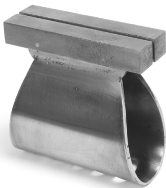
Figure 5. Vice extension, brass (jaws) and steel (spring body), 66 mm high × 69 wide × 31 deep. The vice extension is held in a rougher vice; the cut brass sheets for the plates are hammered over its edges to produce sharp, precise folds.
