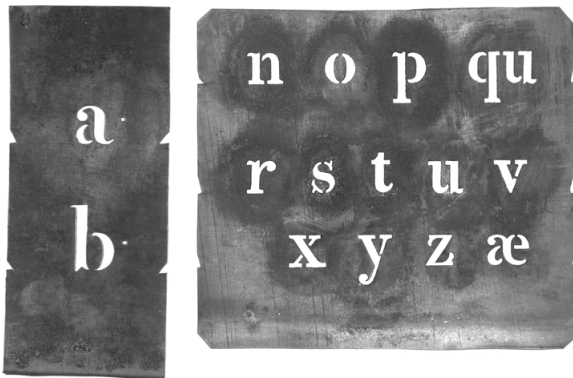
Figure A4.5. Stencil plates, makers not known, French, c. first half of the 19th century, brass, etched; 108×47 mm (left), 88×97 mm (right). Example at right: Abbey of Bellfontaine.
