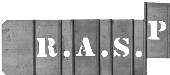
Figure A4.36. Reese's Adjustable Stencil Plates, made by S. W. Reese & Co., United States, based on US Letters Patent no. 148,087 (1874) and no. 173,058 (1876), die-stamped and folded, spring brass, 57×30 mm (R plate). The earliest patent for a 'settable-units' stencil was issued in 1840, in the US. A succession of related patents followed, culminating in the Reese patents of 1874 and 1876 (definitive). This invention, unchanged but now known as 'interlocking stencils', is still in production by the original manufacturer (Hanson). See Kindel (2006).
