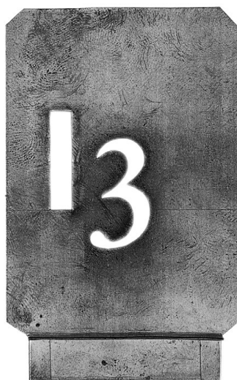
Figure 31. Stencils: multi- and single-part characters with guiding-mark ( repère ) and window ( lumière ) for gauging inter-character space; together with partially and fully stencilled characters; chisel-cut brass. Cut by Fred Smeijers, 2002, based on Des Billettes (c. 1700). All figures actual size.
