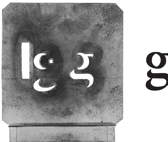
Figure 6. Stencil, cut with short straight chisels and finished with files, brass; and (at right) letter as stencilled. Actual size. Cut by Fred Smeijers, 2002, based on Des Billettes (c. 1700); see also figure 31.
