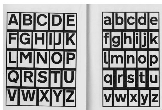
Figure 12. Transport Heavy, for use on signs with white backgrounds. (From Ministry of Transport 1963, pp. 100–101)
